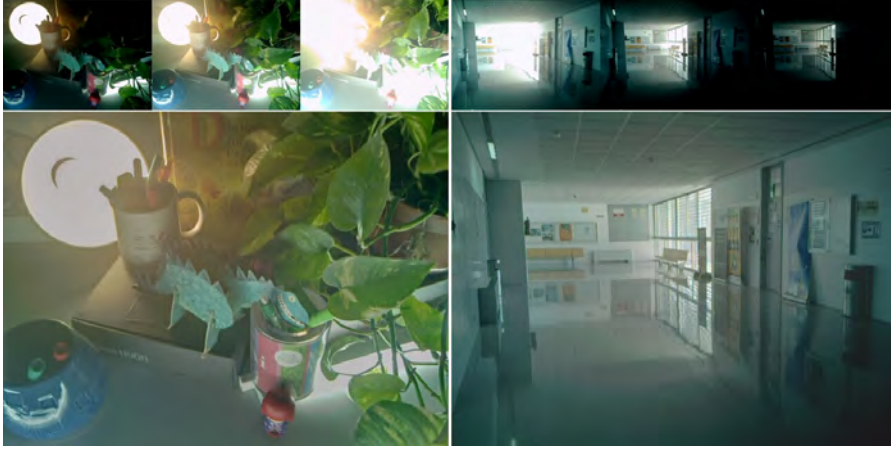
Figure 5.3: Two examples of photos captured and processed by our method. The insets show the bracketed sequence input. The complete pipeline takes less than 20s for a resolution of 640 \times 480 . Left: auto exposure. Right: manual selection of three EVs out of five.
