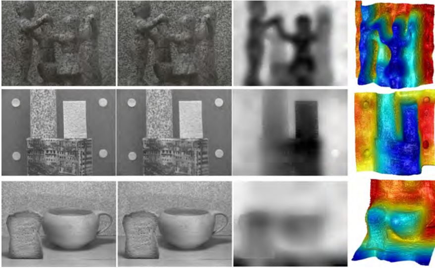
Figure 6.7: Close focus (left), Far focus (middle left), our estimated depth map (middle right), and its corresponding 3D visualization (right). Colors and shading added for a better visualization.
