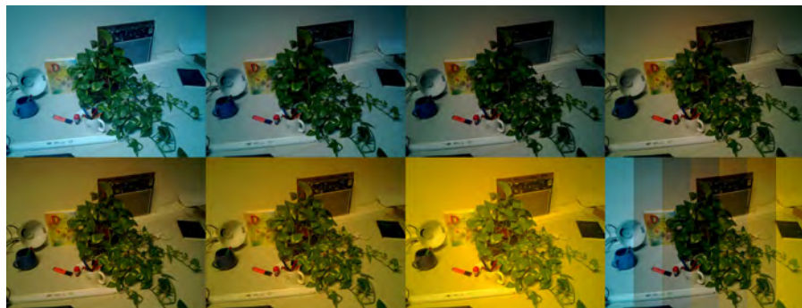
Figure 5.5: From left to right, up to down: sequence of images obtained by capturing the same scene with white balance ranging from 2800K to 11000K. Bottom right shows the selection image presented to the user in order to choose the preferred color temperature.
