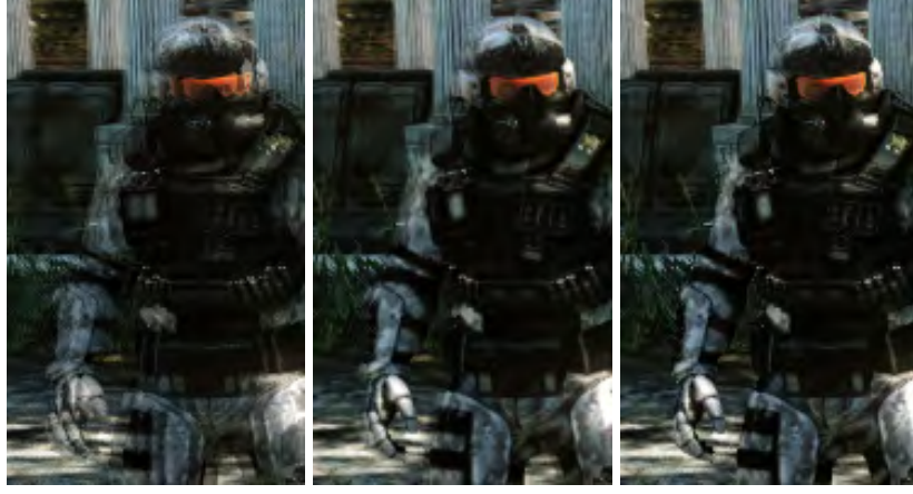
Figure 4.12: Left: Using a naive resolve results in visible ghosting. Middle: Reprojection mitigates these artifacts but does not completely remove them. Right: The addition of velocity weighting allows to completely remove ghosting.
