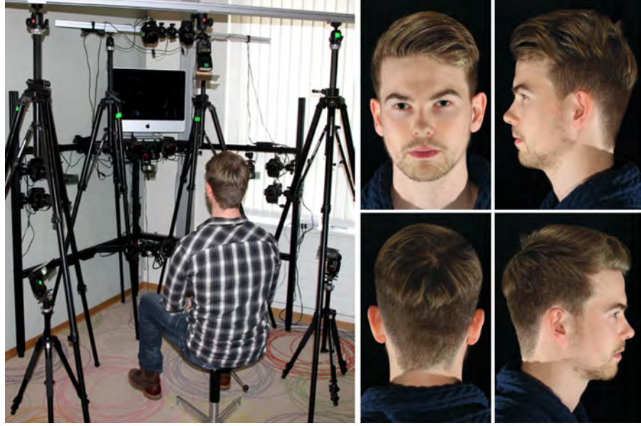
Figure 7.4: Our capture setup consists of 10 cameras placed in a quarter-sphere and we capture 4 different orientations of the subject.
