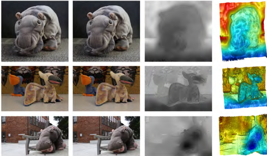
Figure 6.8: Close focus (left), Far focus (middle left), our estimated depth map (middle right), and its corresponding 3D visualization (right). Colors and shading added for a better visualization. The estimated depth map for the top scene used parameters f=24\text{mm} , f/8 , close focal distance of 0.35\text{m} , and far focal distance of 0.75\text{m} . The estimated depth map for the middle scene used parameters f=26\text{mm} , f/8 , close focal distance of 0.4\text{m} , and far focal distance of 0.8\text{m} . The estimated depth map for the bottom scene used parameters f=18\text{mm} , f/8 , close focal distance of 0.5\text{m} , and far focal distance of 15\text{m} .
