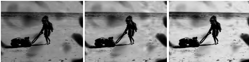
Figure 2.21: From left to right: Exploration of the iodide/bromide ratio parameter with values of 42/60, 70/30 and 100/0 respectively. A higher ratio produces an increase in contrast due to a steeper and shorter spectral sensitivity (Figure 2.7, center) and in final density (as seen in Figure 2.16).
