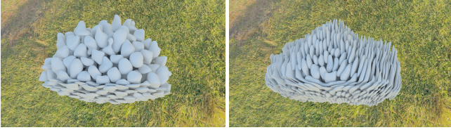
Figure 5: Our framework can generate multiscale granular media with grains in settled positions. In the left image, the generated rockpile shows smaller grains at the bottom and larger ones at the top, with well-defined contact points even across scales. The right image illustrates the same cloud, but with an additional polynomial function applied to the rotation angle, \theta = 15 + p_z , as defined in Eq. 14 of the main document.
