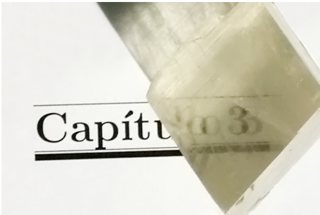
Fig. 1 Light rays split into two by a calcite crystal and forming two images.
