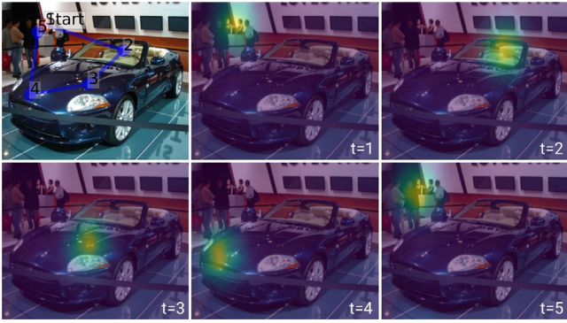
Fig. 3. An example of our spatialized scanpath representation. The top left image shows a RGB image with a sample ground-truth scanpath overlaid. For that sample ground-truth scanpath, we transform each fixation point into a Gaussian map centered at that particular point (see Section 3.1).
