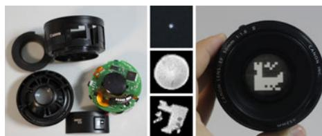
Figure 1: *Left*: Disassembled Canon EOS 50mm f/1.8 used in our tests. *Middle*: Point spread function for different apertures and degrees of defocus (*from top to bottom*: circular aperture, focused; circular aperture, defocus depth = 90cm; and one of our coded apertures, defocus depth = 80cm). *Right*: The lens with one of our coded apertures inserted.
