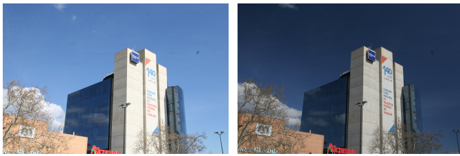
Fig. 1: Real photographs obtained with different polarization filters. Left image is an image without any polarizer and right image with a linear polarizer, where the sky tone has notorious changes, modifying the saturation. Another common use of polarizers is to modify the reflections on different specular surfaces.
