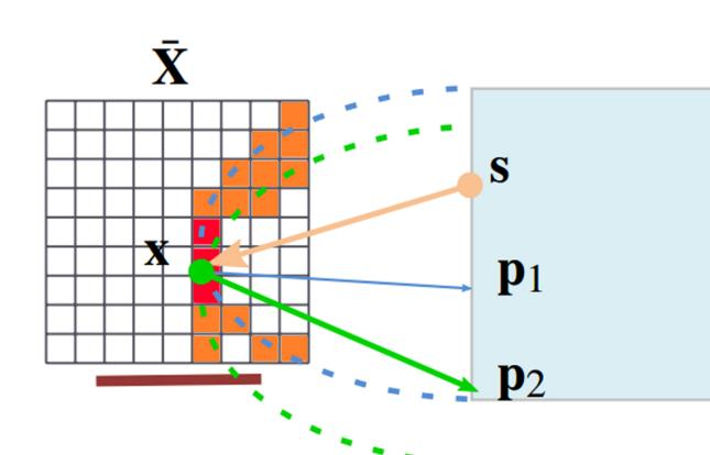
1 The intersection of several of these ellipsoids defines a probability map for the occluded geometry without need of individual per-voxel computations
