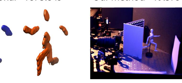
← Reconstruction of a real mannequin using a streak camera and a femtosecond laser (depicted at bottom-right), using traditional backprojection (left) and our method (right). We achieve a **speed-up of** two orders of magnitude while obtaining similar reconstruction quality. from Data and inset [Velten 2012]
