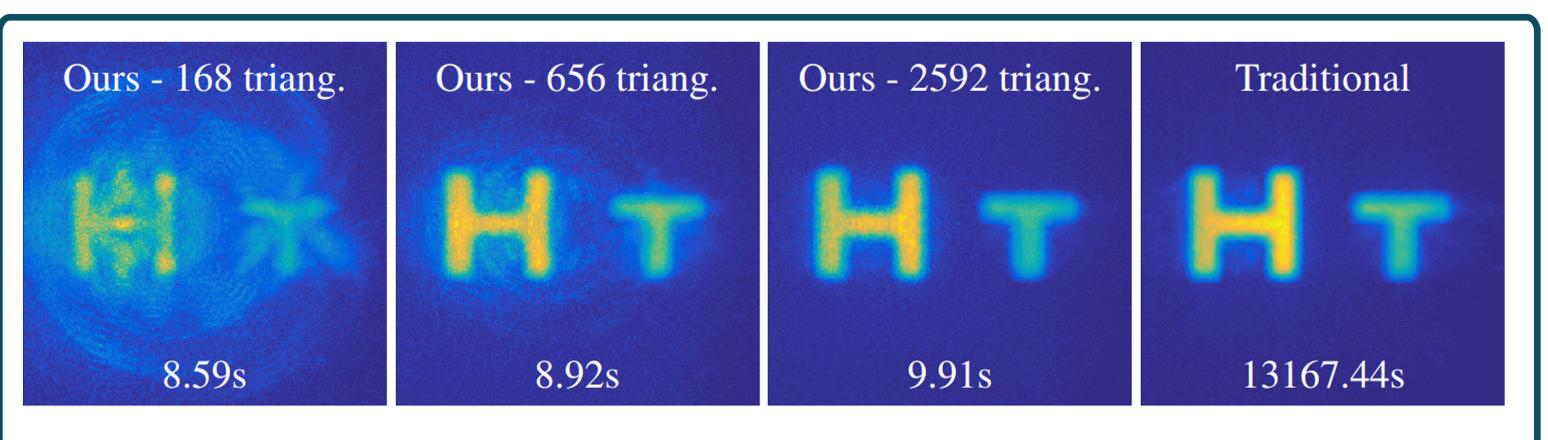
1 Reconstruction of a synthetic scene rendered with [Jarabo 2014] for various tesellation quality levels. Right: The same synthetic scene reconstructed using traditional backprojection. As we can see, not only our method offers indistingishable results from traditional backprojection while offering a speed-up of more than 1300x, but also we are able, unlike current state-of-the-art approaches, to trade quality for computation time as desired by adjusting the tesellation levels used.
