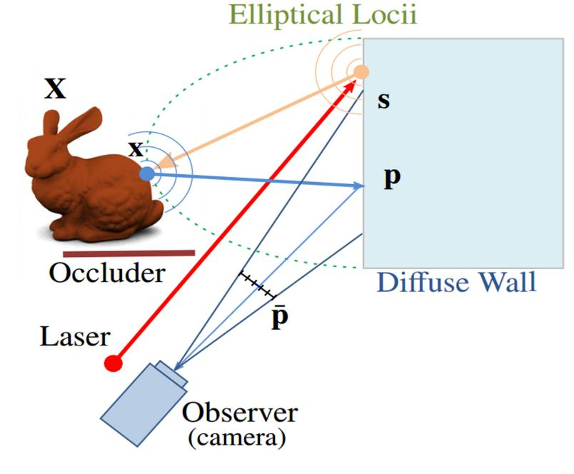
A laser pulse is emitted towards a diffuse wall, creating a virtual point light **s** illuminating the occluded scene X. The reflection of the occluded geometry travels back to the diffuse wall, which is imaged by the camera.
