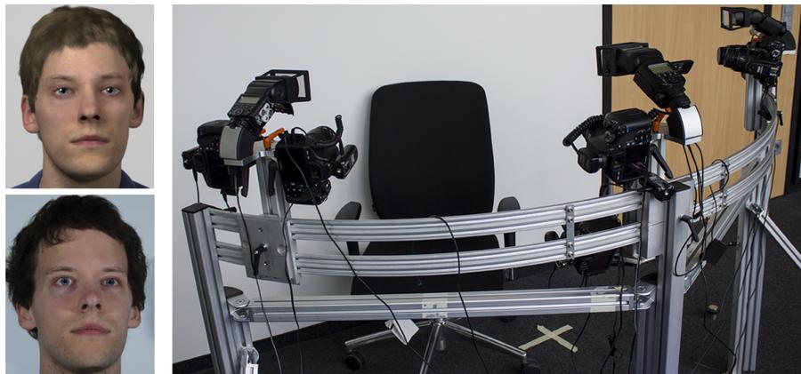
Figure 8: Our face scanning setup (right) and comparison between photographs and virtual reconstructions of our actor (left).
