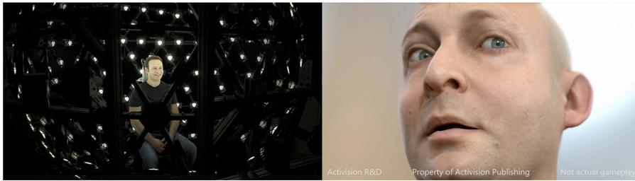
Figure 2: Light Stage used for capturing the appearance of a real human, rendered on the right in real time. Images from *USC Institute for Creative Technologies* and *Activision RD* [7].
