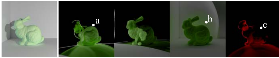
Figure 5.16: Fluorescent bunny illuminated by a pulse of light from a point light source. Light reaches the bunny, which reflects light centered in the green-ish spectra (b), and the rest is absorbed. After 10 ns, part of the absorbed light gets re-emitted at lower quantum energy, centered at 680 nm (c). Because of this re-emission, the hue of the bunny in steady state (a) is shifted towards yellow.
