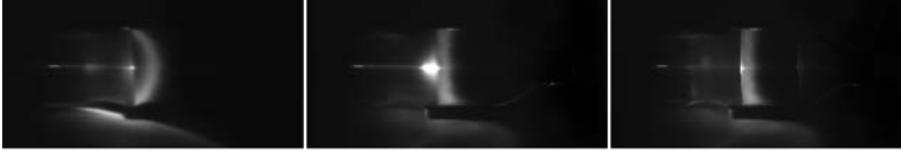
Figure 4.9: Time unwarping for the bottle scene, containing a scattering medium. From left to right: a frame of the video without correction, where the energy front appears curved; the same frame after time-unwarping with respect to distance to the camera z_{ij} ; the shape of the energy front is now correct, but it still appears before the pulse; the same frame, time-unwarped taking also scattering into account.
