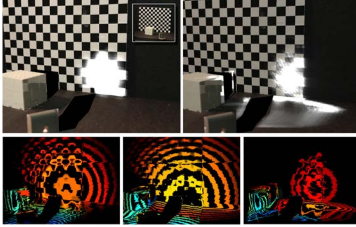
Figure 6.2: Time unwarping between camera time and world time for synthesized new views of a cube scene. Top row, left: Scene rendered from a novel view keeping the unwarped camera time from the first frame (the small inset shows the original viewpoint). Right: The same view, warping data according to the new camera position. Notice the large changes in light propagation, in particular the wavefronts on the floor not visible in the previous image. Bottom row: Isochrones visualization of the cube-scene for a given virtual camera (color encodes time); from left to right: original x-y-t volume in the time-frame of the capturing camera, unwarped x-y-t data in world time frame, and re-warped data for the new virtual camera.
