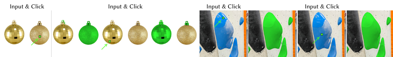
Fig. 7. Our method can differentiate between materials with the same albedo and different roughness (left columns), but sometimes struggles when the differences are too subtle and appear within an object (right columns), presumably since these cases are under-represented in our training dataset.
