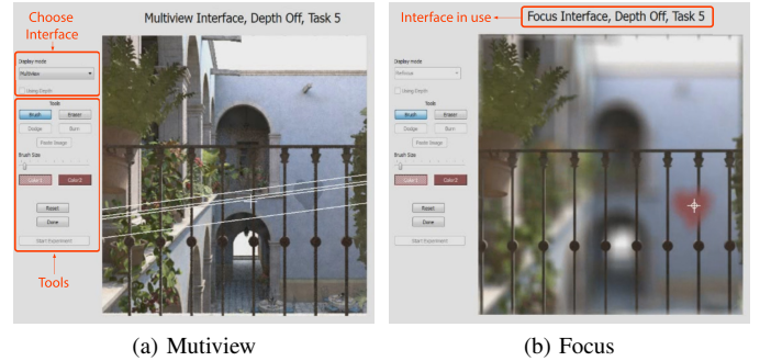
Fig. 4: User interfaces used in our tests. In the Multiview paradigm, epipolar lines (white) mark the trajectory a currently active stroke will follow when moved in depth. In the Focus paradigm, the in-focus plane marks the depth at which strokes will be placed.
