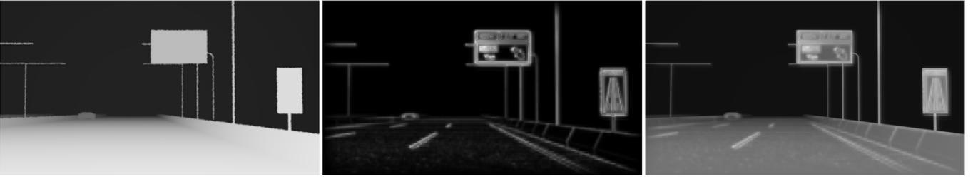
Figure 2: The three maps computed for the Road scene in Figure 9: the X-map (left), the saliency map (center) and the XS-map (right).
